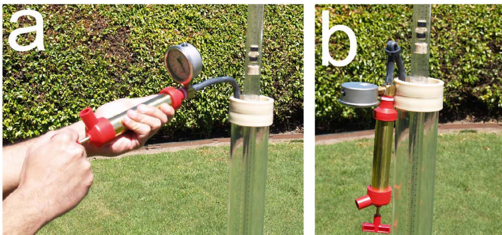
Fig. 36. Applying vacuum to Reservoir.
