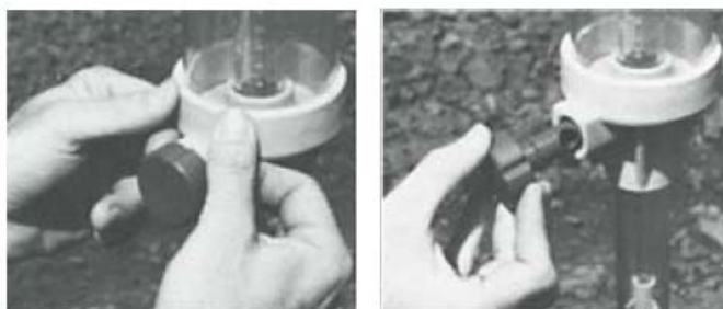
Fig. 37. Removing Reservoir Valve.
